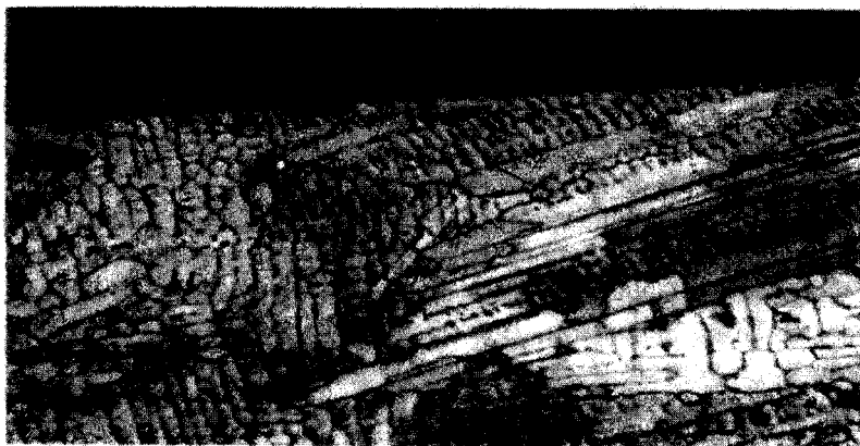
Figure 1 - Structure of a Cast Lead - 0.75% Ag Anode (magnification 160x)
