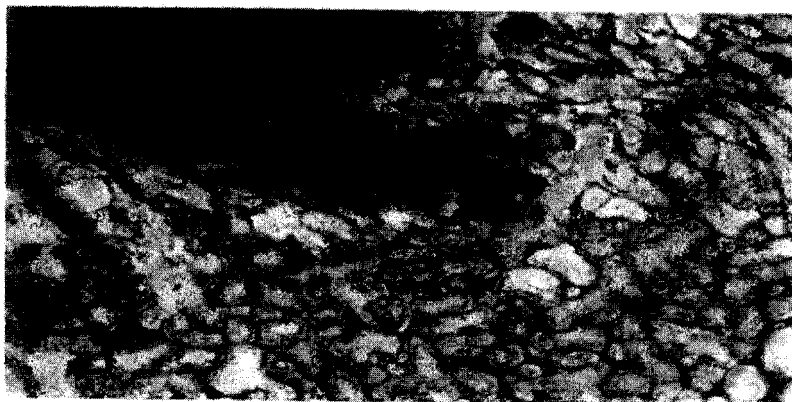
Figure 2 - Defects in a Cast Pb - 0.75% Ag Anode (magnification 320x)
