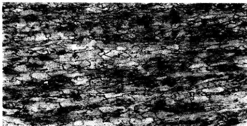
Figure 6 - Grain Structure of a Rolled Pb-Ca-Ag Anode (magnification 160x)
