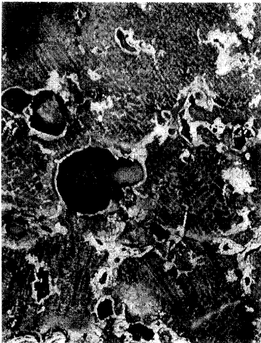
Figure 1 - Cast Pb-Ca-Sn alloy anode cross section. Note air bubbles and dross (oxides) trapped in the metal.
